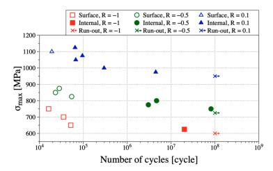
**Figure 2.** Relationship between the maximum applied stress and the number of cycles to fracture for different stress ratios. A step-wise shape is observed for the stress ratios R = -1 and R = -0.5, but an asymptotic shape is observed for R = 0.1.
