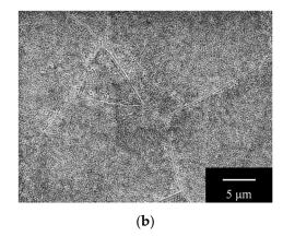
**Figure 1.** Microstructure of the applied Ti-22V-4Al alloy with a homogenous and fine α-phase precipitation from SEM analysis: (a) low-magnification and (b) high-magnification images. The material was polished to a mirror finish and then etched with Kroll's reagent (HF:HNO<sub>3</sub>:H<sub>2</sub>O = 1:2:50) for 8–10 s.
