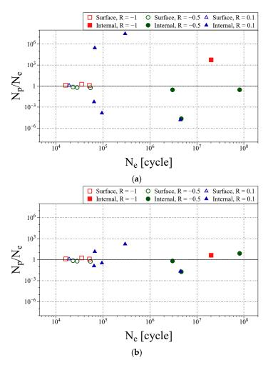
**Figure 13.** Relationship between the predicted and experimental fatigue life  $(N_p/N_e)$ . (a) Using total facets area; (b) Using major facet area.
