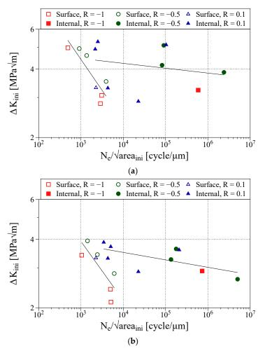
**Figure 12.**  $\Delta K_{ini} - N_e / \sqrt{area_{ini}}$  diagrams. (a) Total facets area (surface:  $C = 5.04 \times 10^{-9}$ , m = 3.68; internal:  $C = 2.1 \times 10^{-38}$ , m = 46.7); (b) Major facet(s) area (surface:  $C = 5.76 \times 10^{-9}$ , m = 3.84; internal:  $C = 1.72 \times 10^{-25}$ , m = 30.5).
