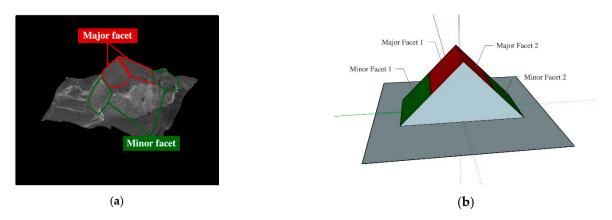
**Figure 11.** Example of the combination type. These facets are the same facets shown in Figure 7b ( $\sigma_{max} = 625$  MPa, R = -1,  $N_{\rm f} = 2.0 \times 10^7$ ). (a) 3D-SEM image; (b) 3D-model schematic image.
