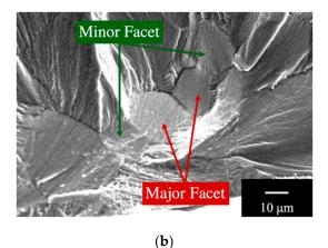
**Figure 7.** SEM images of the multiple facets under negative stress ratios. (a)  $\sigma_{max} = 800$  MPa, R = -0.5,  $N_{\rm f} = 4.7 \times 10^6$ ; (b)  $\sigma_{max} = 625$  MPa, R = -1,  $N_{\rm f} = 2.0 \times 10^7$ .
