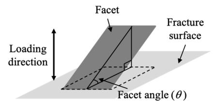
Figure 4. Schematic of the facet angle measurement.
