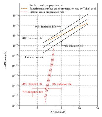
**Figure 15.** Relationship between crack propagation rate and stress intensity factor range derived from the Tanaka-Akiniwa model in terms of fracture mode and crack initiation life.
