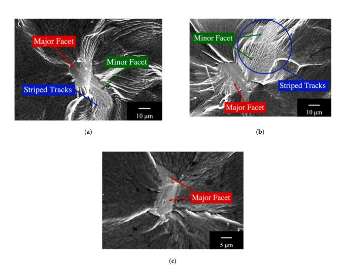
**Figure 6.** SEM images of the multiple facets under positive stress ratio. (a)  $\sigma_{max} = 1125 \text{ MPa}$ , R = 0.1,  $N_{\rm f} = 6.5 \times 10^4$ ; (b)  $\sigma_{max} = 975 \text{ MPa}$ , R = 0.1,  $N_{\rm f} = 4.5 \times 10^6$ ; (c)  $\sigma_{max} = 1000 \text{ MPa}$ , R = 0.1,  $N_{\rm f} = 3.0 \times 10^5$ .
