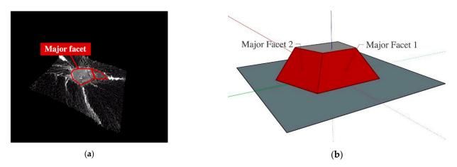
**Figure 10.** Example of the peak type. These facets are the same facets shown in Figure 6c ( $\sigma_{max} = 1000$  MPa, R = 0.1,  $N_f = 3.0 \times 10^5$ ). (a) 3D-SEM image; (b) 3D-model schematic image.
