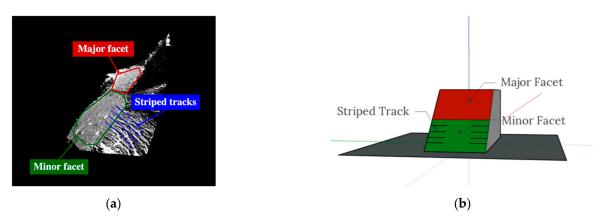
**Figure 8.** Example of the vertical slope type. These facets are the same facets shown in Figure 7a ( $\sigma_{max} = 800$  MPa, R = -0.5,  $N_f = 4.7 \times 10^6$ ). (a) 3D-SEM image; (b) 3D-model schematic image.
