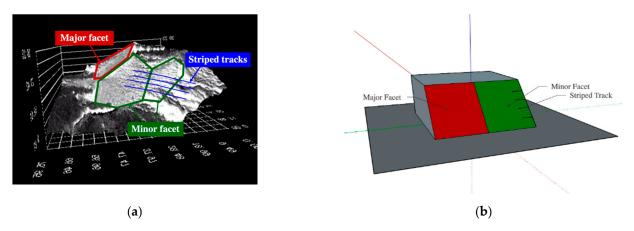
**Figure 9.** Example of the horizontal slope type. These facets are the same facets shown in Figure 6b ( $\sigma_{max} = 975 \text{ MPa}$ , mboxemphR = 0.1,  $N_f = 4.5 \times 10^6$ ). (a) 3D-SEM image; (b) 3D-model schematic image.
