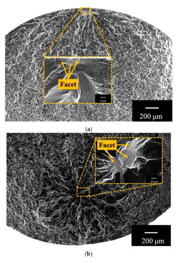
**Figure 3.** SEM images of the fracture surface. (a) Surface fracture,  $\sigma_{max} = 700$  MPa, R = -1,  $N_{\rm f} = 3.5 \times 10^4$ ; (b) Internal fracture,  $\sigma_{max} = 975$  MPa, R = 0.1,  $N_{\rm f} = 4.5 \times 10^6$ .
