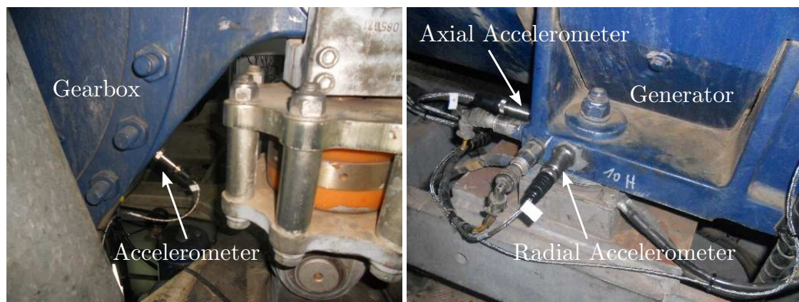
Figure 4. The radial vibration sensor installed near the planetary gear on the left and both axial and radial vibration sensors installed on the generator drive end on the right.
