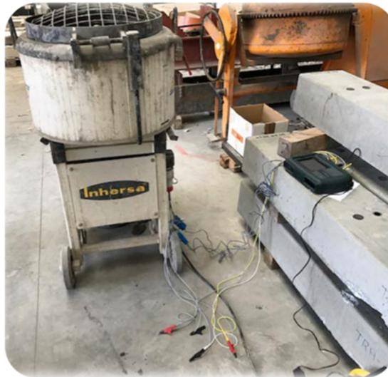
**Figure 6.** Instrument-fitted concrete mixer.
