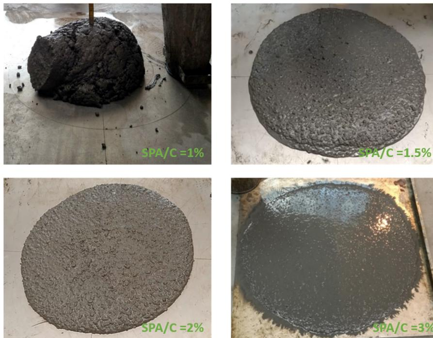
Figure 10. Detail of slump flow test.
