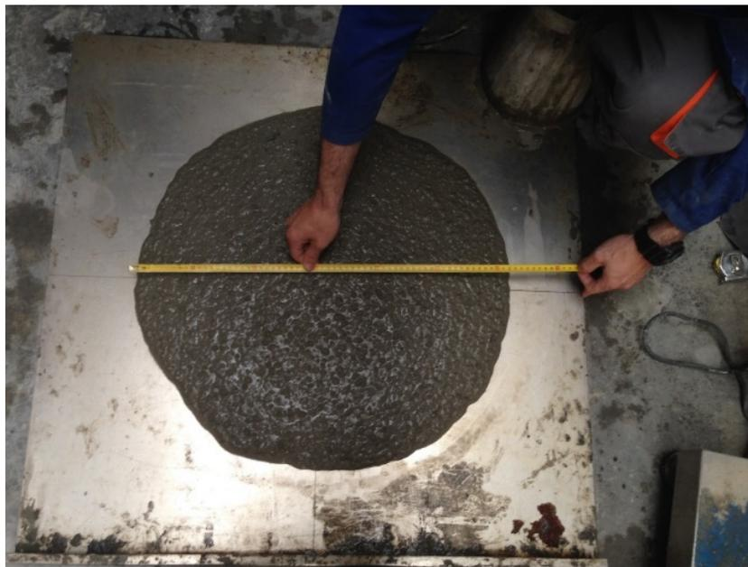
**Figure 3.** Slump flow test diameter measurement example.
