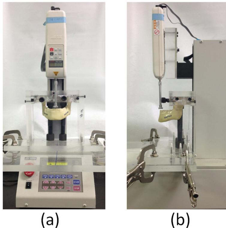
**Figure 2.** Artificial mandibular bone fixed to a supporting base for the biomechanical test: (a) frontal view; (b) side view.
