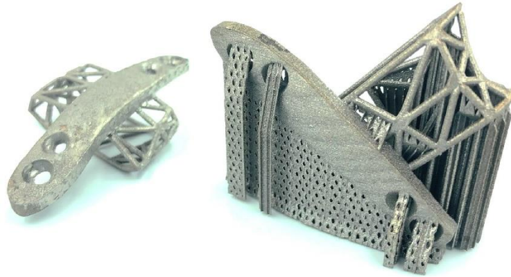
Figure 7. The additively manufactured titanium implant with the supports (right) and without the supports (left).
