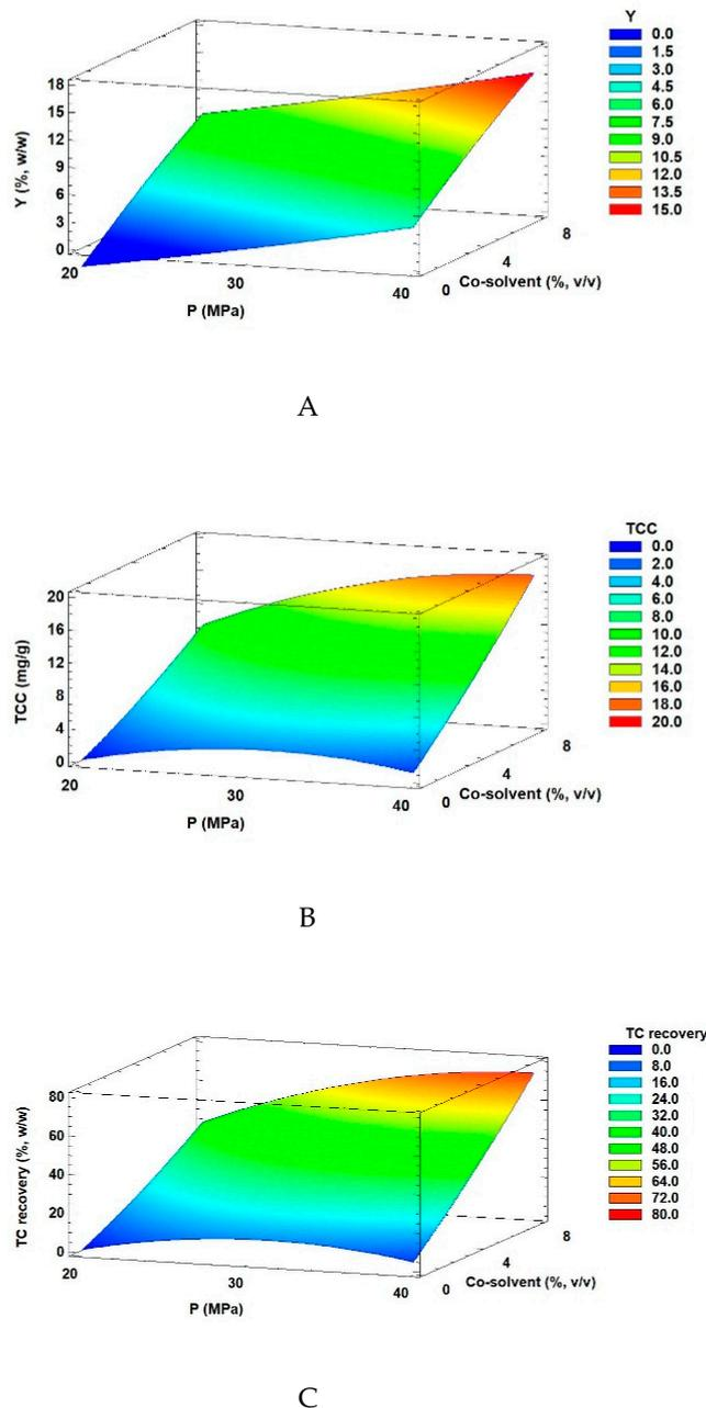
**Figure 3.** Response surface plot showing combined effects of pressure and co-solvent on (A) extraction yield (Y), (B) total carotenoids content (TCC), and (C) recovery (TC recovery) from *I. galbana*. All extractions were done at 60 °C temperature.
