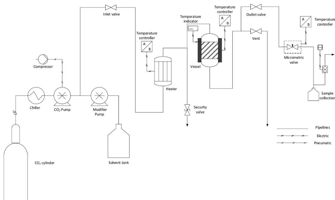
**Figure 1.** Diagram of the supercritical fluid extraction (SFE) equipment (Applied Separations, Speed, Allentown, PA, USA). The main parts are: CO<sub>2</sub> cylinder; CO<sub>2</sub> pump; compressor; modifier pump; solvent tank; inlet valve; heater; extraction vessel and oven vessel; micrometric valve; sample collection.
