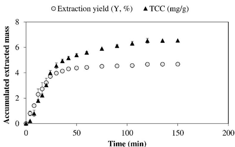
**Figure 2.** Kinetics of improving extraction yield (Y, %) and total carotenoids content (TCC) from *I. galbana* during 150 min. The working conditions were at the central point: 50 °C, 30 MPa, 4% co-solvent (ethanol, v/v), and a CO<sub>2</sub> flow rate of 7.2 g/min.
