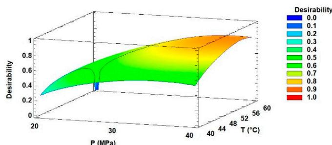
**Figure 6.** Surface of the desirability function in terms of pressure, temperature and maximum co-solvent (8% ethanol, v/v) obtained for maximizing extraction yield (Y), total carotenoids content (TCC) and recovery (TC recovery), phenol content (TPC), TEAC method, and FAMEs content from *I. galbana*.
