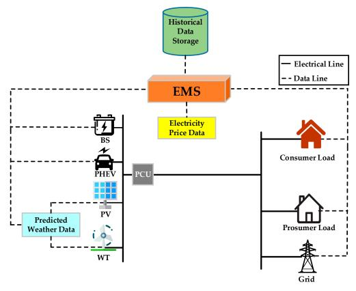
Figure 1. Proposed energy system architecture.
