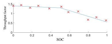
**Figure 7.** Relationship curve between  $\mu_{soc}$  and state of charge (SOC).
