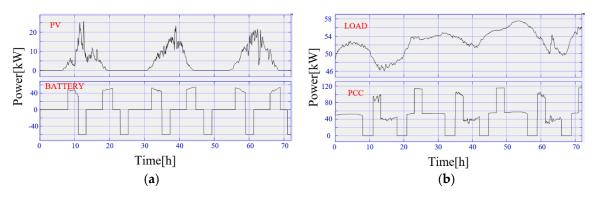
Figure 11. Waveforms of Scene 2: (a) PV and storage; (b) load and PCC.
