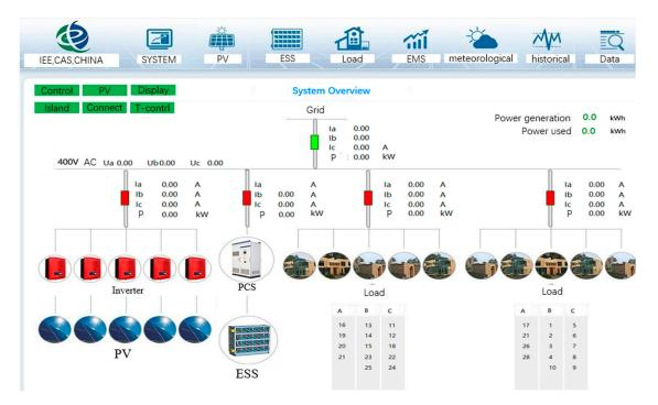
Figure 26. Interface of the monitoring system.
