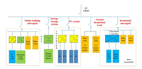
Figure 2. System structure diagram of the community microgrid.
