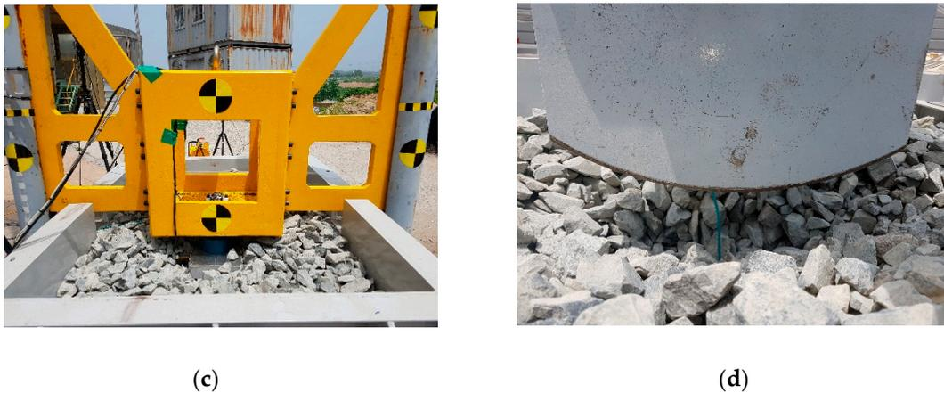
**Figure 8.** Drop test to simulate the collision between the dropped weight and gravel layer: (a) Front view of the drop test; (b) gravel layer; (c) weight penetration; (d) gravel layer after penetration.
