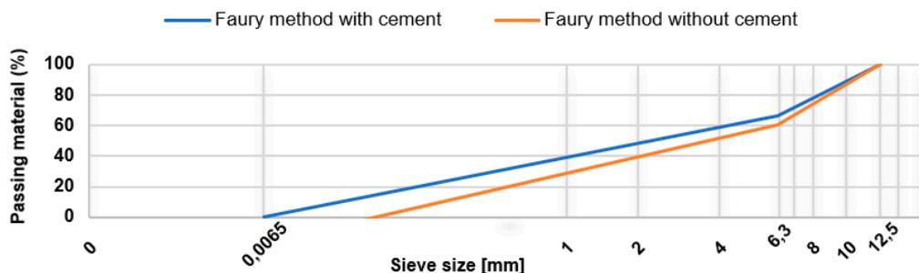
Figure 1. Faury method for reference concrete.
