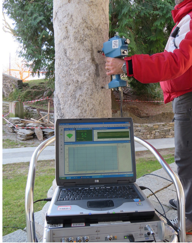
Figure 5. Setup of the impact test.
