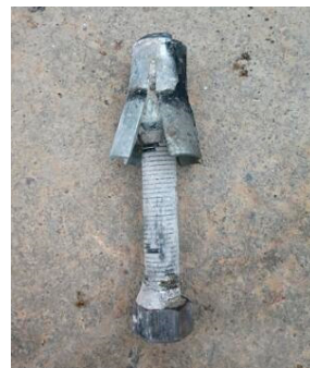
Figure 8. Embedded extension of blind bolt.
