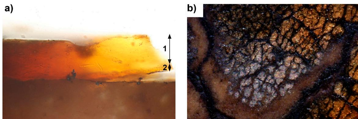
**Figure 3.** VIS-light image of a painting sample as seen under Optical Microscopy (OM): (a) cross-section of the gilded surface; (b) surface with the varnished (yellow) and unvarnished (gray) silver (Ag) layer.
