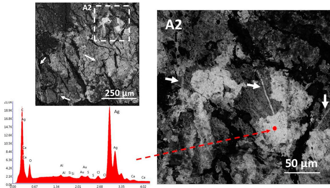
**Figure 7.** SEM-BSE images of the surface of the untreated painting sample. A SEM-EDS analysis was carried out on the silver leaf.
