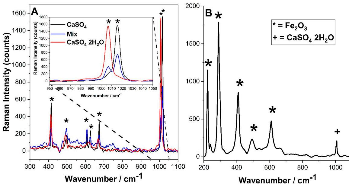
**Figure 10.** Raman spectra acquired on the ground of the painting cross-section: (A) Raman spectra acquired on white grains (B) Raman spectrum acquired on red grains.
