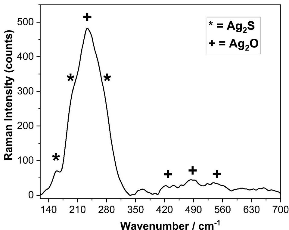
Figure 9. Raman spectrum acquired on the silver layer of the painting cross-section.
