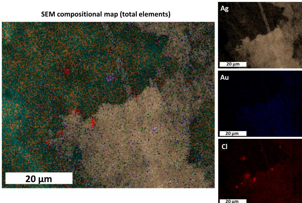
**Figure 8.** SEM-EDS elemental map of the surface A2 shown in Figure 7.
