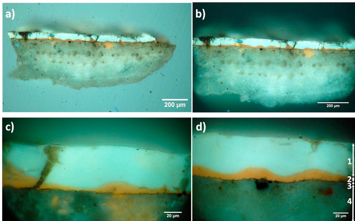
**Figure 2.** UV fluorescence microscope images of a painting cross-section at different magnification objectives: (a) 10 $\times$ , (b) 20 $\times$ , and (c,d) 100 $\times$ . Four different layers were observed: (1) a white-opalescent layer (circa 40  $\mu$ m); (2) an orangish layer (circa 15  $\mu$ m); (3) a sub-micron black layer; and (4) a very thick whitish preparation layer.
