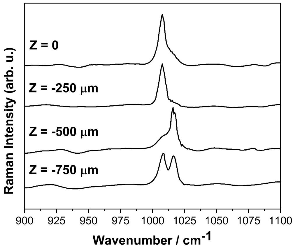
**Figure 11.** Raman spectra acquired at different depth (Z) on the ground of the painting cross-section. Z = 0 corresponds to the surface underneath the Ag layer.
