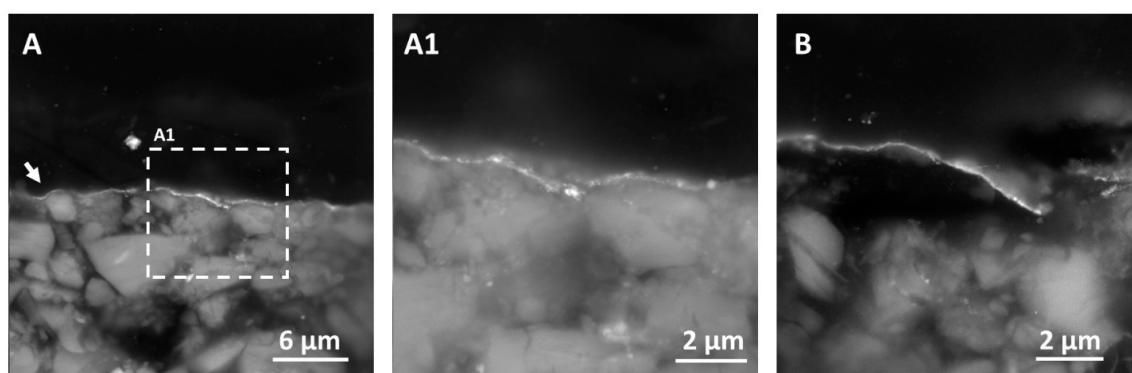
**Figure 6.** SEM-BSE images of the silver leaf. Figure A and B show the silver leaf in two different areas of the cross-section. Figure A1 shows a magnified view of the area inside the white-dashed square in figure A.
