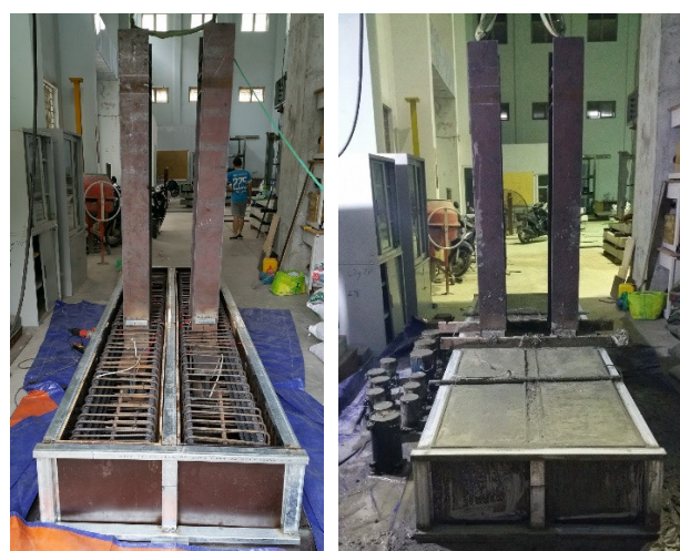
Figure 3. Casting of the specimens.
