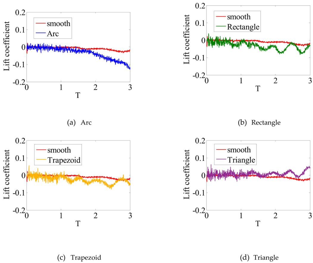
**Figure 13.** The comparison of the lift coefficients between the smooth cylinder and cylinder with strips of different shapes for  $Re = 55,000$ .
