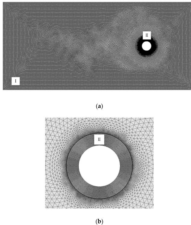
**Figure 2.** Sketch of the computational domain (I is the dynamic mesh zone; II is the accompanying moving zone): (a) the whole computational zone; (b) the mesh near the cylinder.
