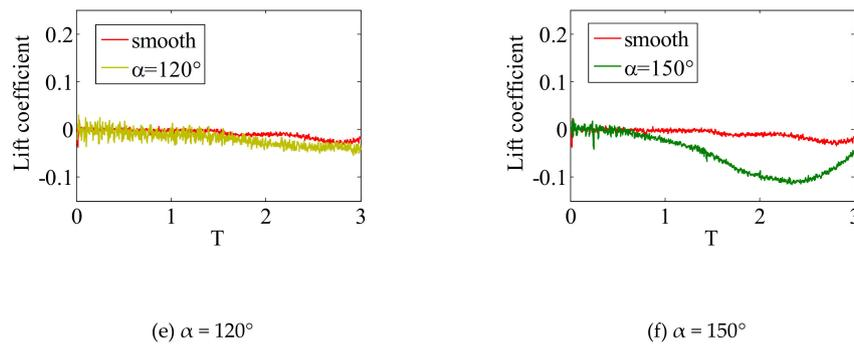
**Figure 8.** The comparison of the lift coefficients between the smooth cylinder and cylinder with strips for  $Re = 55,000$ .
