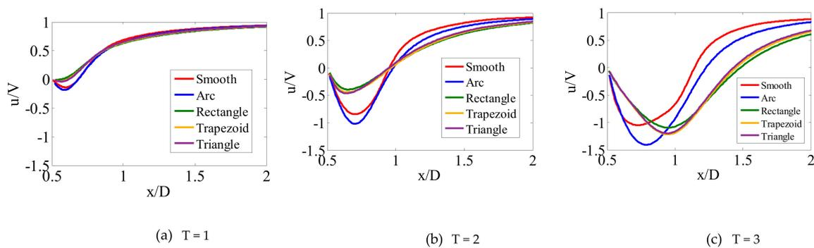
**Figure 16.** The comparison of the velocity distribution at different moments on the axis between the smooth cylinder and cylinder with strips of different shapes for  $Re = 55,000$ .
