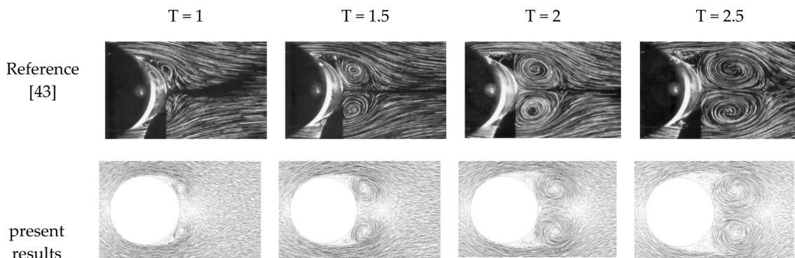
Figure 4. The comparison of the wake flow between the present solutions and the results of Reference [43] for  $Re = 5000$ .
