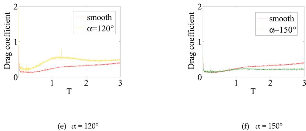
**Figure 7.** The comparison of the drag coefficients between the smooth cylinder and cylinder with strips for  $Re = 55,000$ .
