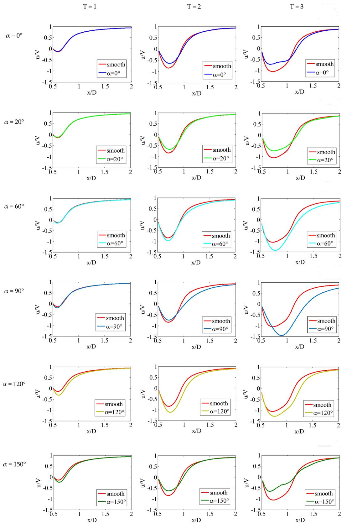
**Figure 11.** The comparison of the velocity distribution at different moments on the axis between the smooth cylinder and cylinder with strips for  $Re = 55,000$ .
