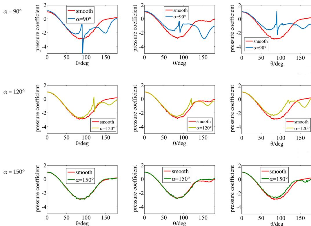
**Figure 10.** The comparison of the pressure coefficient between the smooth cylinder and cylinder with strips for  $Re = 55,000$ .
