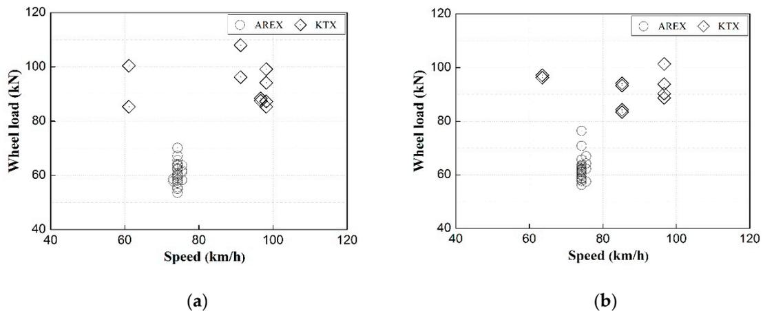
Figure 4. Measured dynamic wheel load by train type. (a) Before rail pad replacement and (b) after rail pad replacement.
