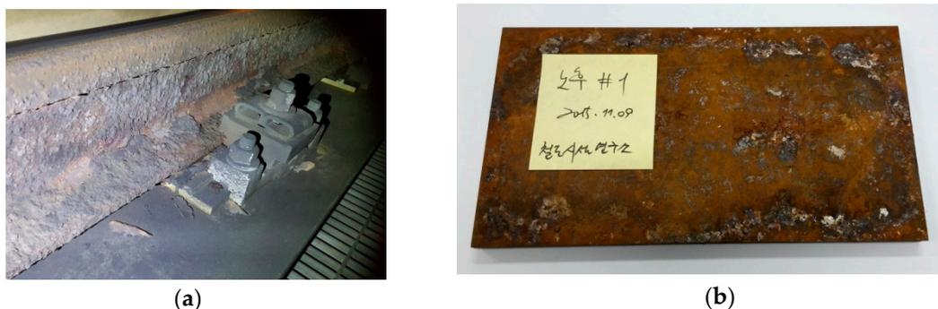
**Figure 2.** Photographs of corroded rail and pad. (a) Corroded track components and (b) corroded rail pad.
