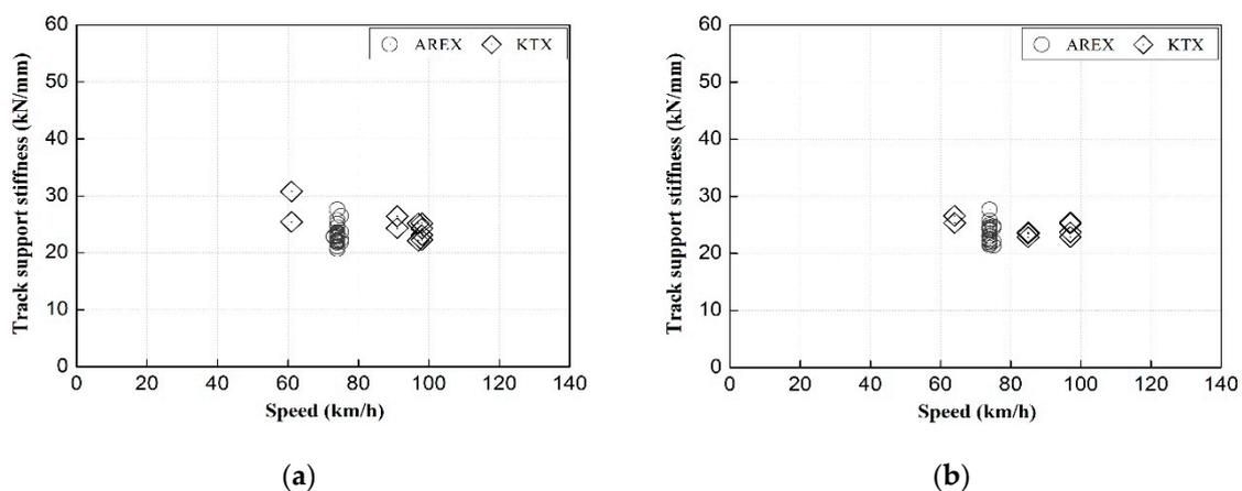
**Figure 15.** Calculated track support stiffness according to train type (including the track girder bending stiffness). (a) Before rail pad replacement and (b) after rail pad replacement.
