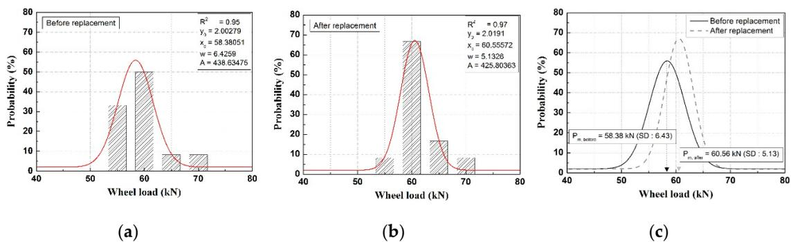
Figure 5. Comparison of the measured dynamic wheel load according to rail pad replacement. (a) Before rail pad replacement; (b) after rail pad replacement; and (c) dynamic wheel load fluctuation for before and after rail pad replacements.
