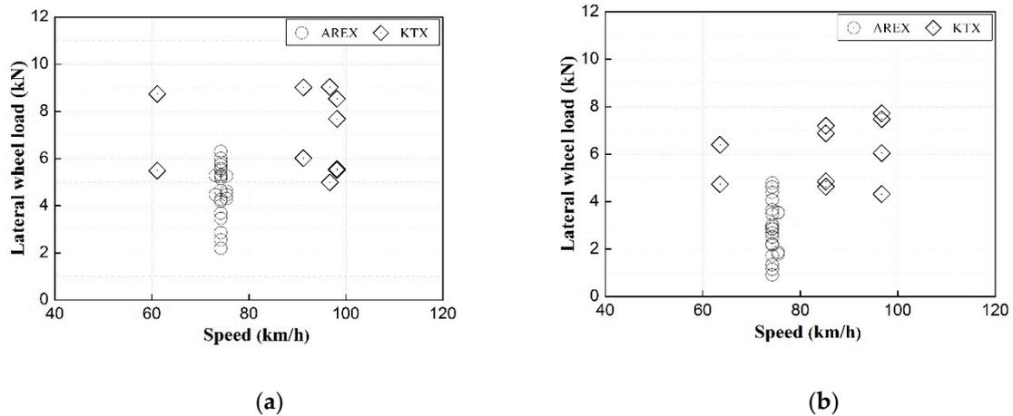
**Figure 6.** Measured lateral wheel load by train type. (a) Before rail pad replacement and (b) after rail pad replacement.
