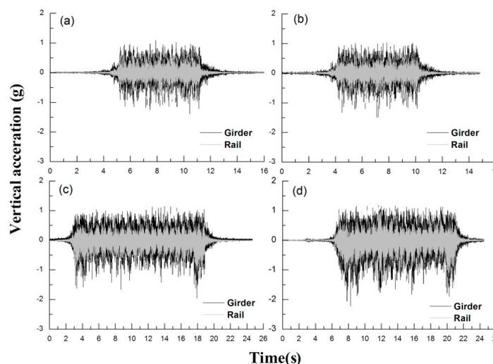
**Figure 12.** Comparison of the measured vertical acceleration of the rail and track girder. (a) Before rail pad replacement for AREX; (b) after rail pad replacement for AREX; (c) before rail pad replacement for KTX; and (d) after rail pad replacement for KTX.
