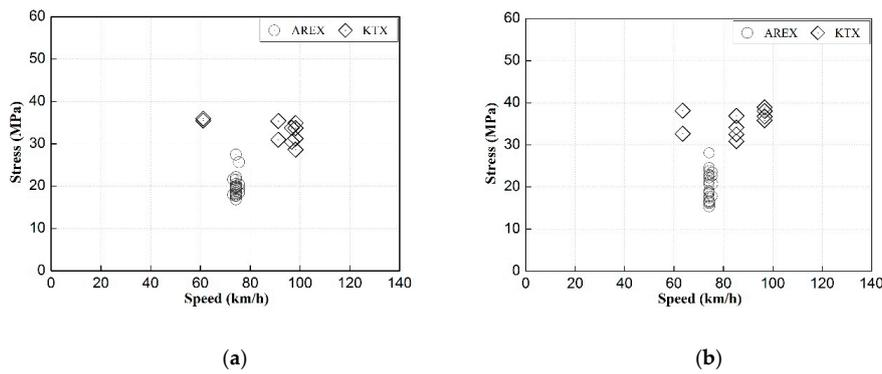
**Figure 11.** Measured bending stress of the rail by train type. (a) Before rail pad replacement and (b) after rail pad replacement.
