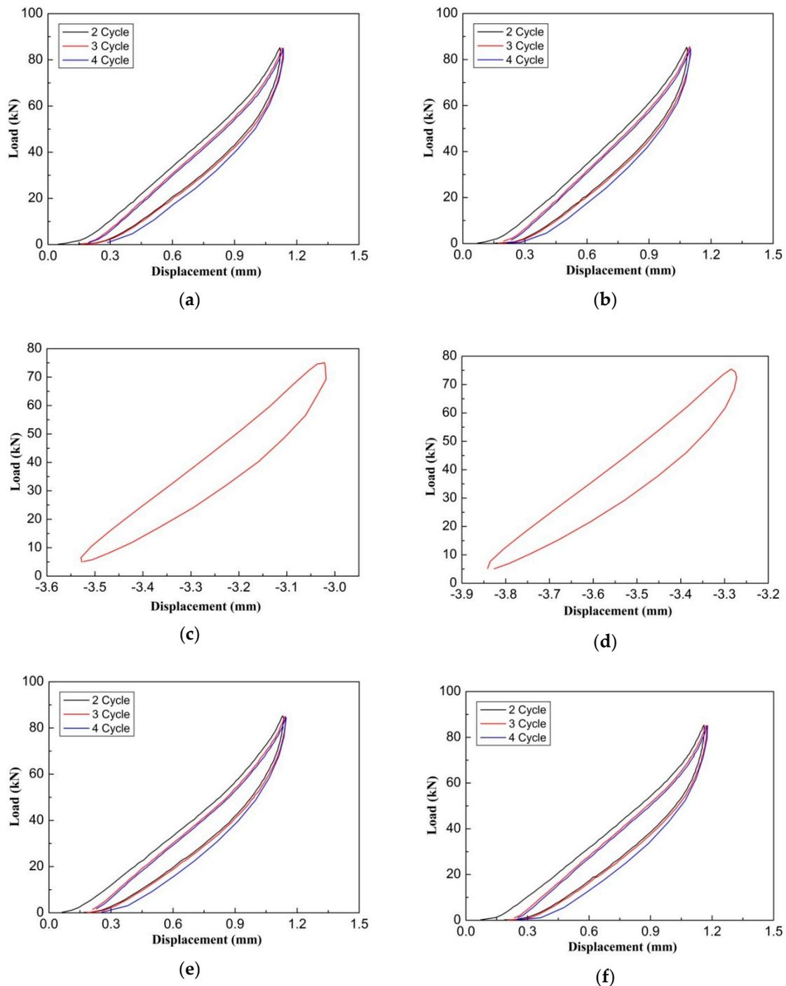
**Figure 18.** Load–displacement curves. (a) Static test (new rail pad); (b) static test (used rail pad); (c) dynamic test (new rail pad); (d) dynamic test (used rail pad); (e) static test after aging tests (new rail pad); and (f) static test after aging tests (used rail pad).
