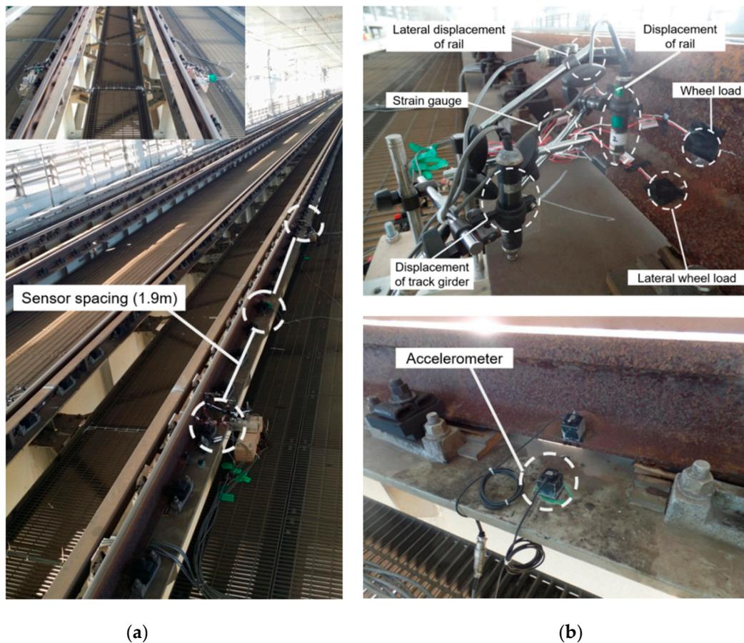
**Figure 3.** Sensor installation. (a) Location of the measurement and (b) vertical and lateral wheel load strain gauges, strain gauges, vertical rail, and track girder displacements measured using displacement transducers mounted on a jig anchored at the side bridge inspection passage, which is not affected by the passing train [2].
