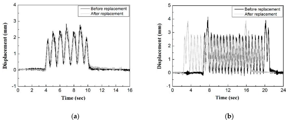
**Figure 7.** Examples of measured vertical displacements of the track girder before and after rail pad replacement. (a) AREX and (b) KTX.
