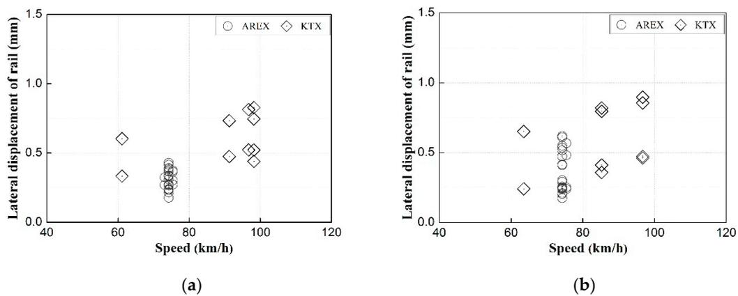
**Figure 10.** Measured lateral displacement of the rail by train type. (a) Before rail pad replacement and (b) after rail pad replacement.
