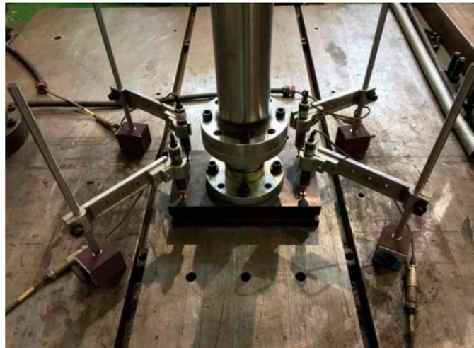
**Figure 17.** Photograph of the rail pad spring stiffness test apparatus.
