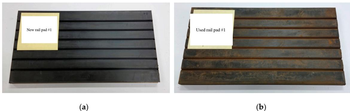
**Figure 16.** Rail pad samples. (a) New rail pad and (b) used rail pad (corroded rail pad).
