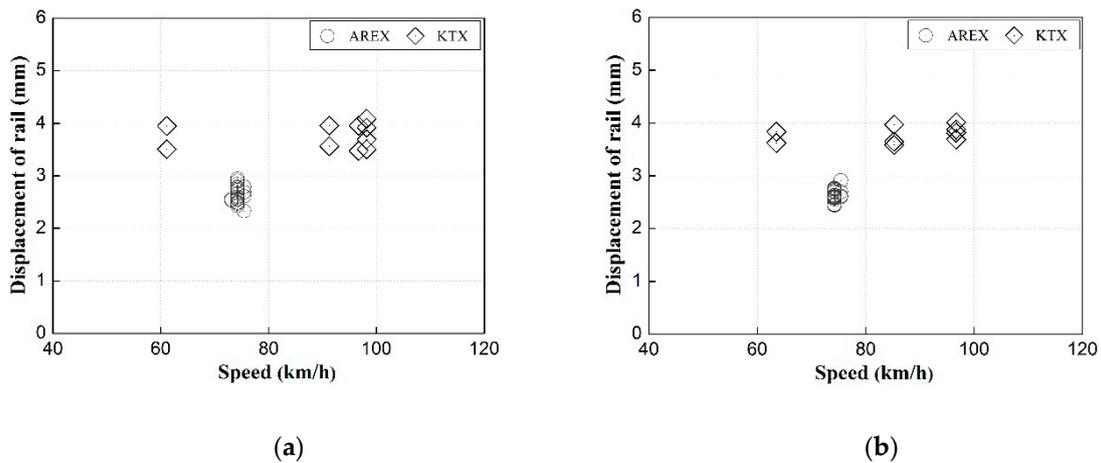
**Figure 8.** Measured displacement of the rail by train type. (a) Before rail pad replacement and (b) after rail pad replacement.
