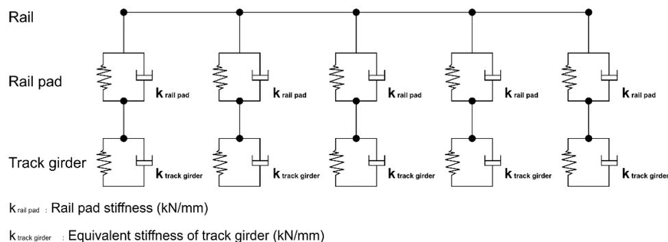
Figure 13. Spring stiffness model of a direct fixation track at the rail supporting points [2].
