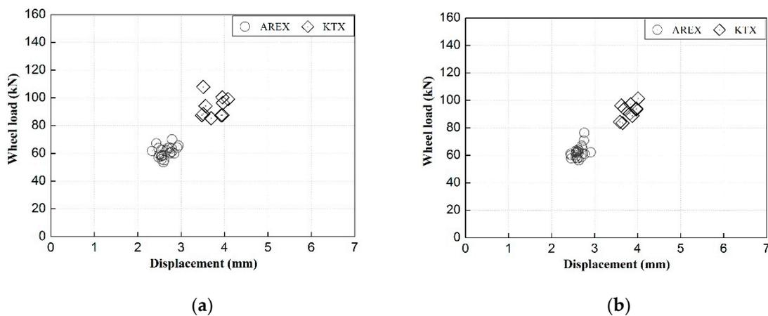
**Figure 14.** Measured wheel load–track displacement according to train type. (a) Before rail pad replacement and (b) after rail pad replacement.
