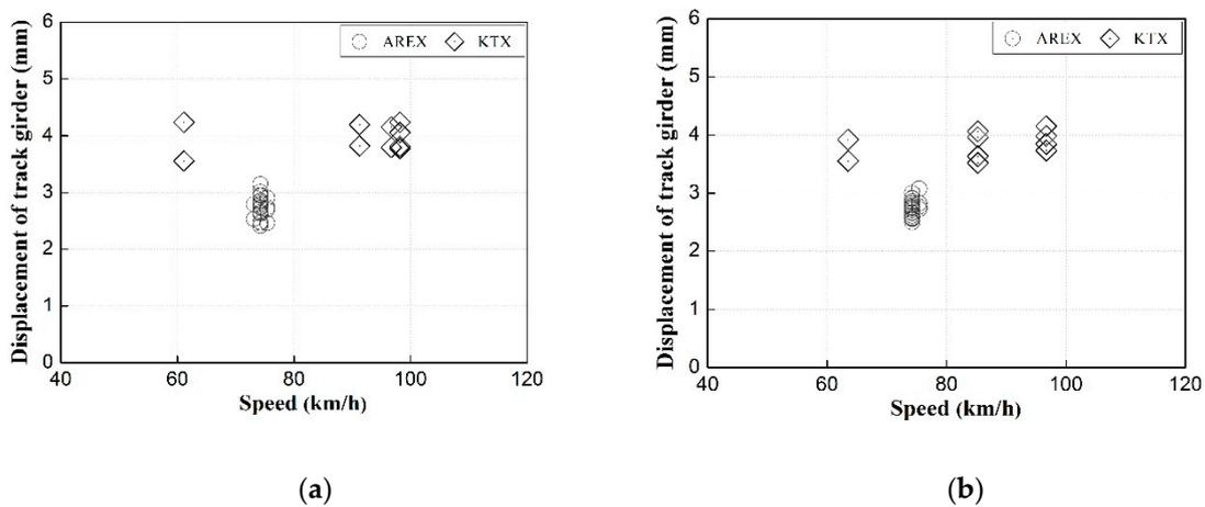
**Figure 9.** Measured displacement of the track girder by train type. (a) Before rail pad replacement and (b) after rail pad replacement.
