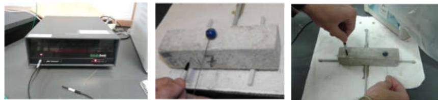
Figure 2. GrindoSonic MK5 equipment (left); test to obtain flexural vibration frequency (center); test to obtain torsional vibration frequency (right).
