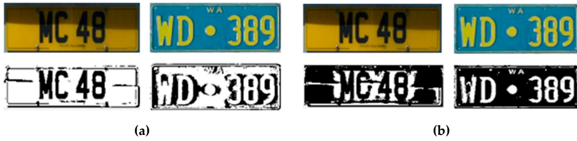
Figure 6. Effectiveness of prior knowledge of FG polarity: (a) License plate (LP) image with dark foreground polarity, (b) LP image with bright foreground polarity.
