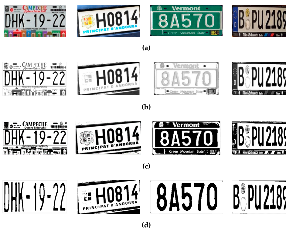
Figure 7. FG polarity uniformity and region of interest (ROI) extraction process: (a) original LP images, (b) gray images, (c) thresholded images, (d) extracted ROI having the same foreground polarity.
