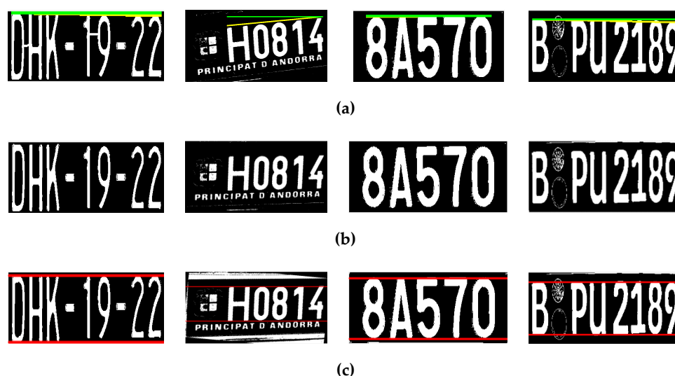
Figure 7. FG polarity uniformity and region of interest (ROI) extraction process: (a) original LP images, (b) gray images, (c) thresholded images, (d) extracted ROI having the same foreground polarity.
