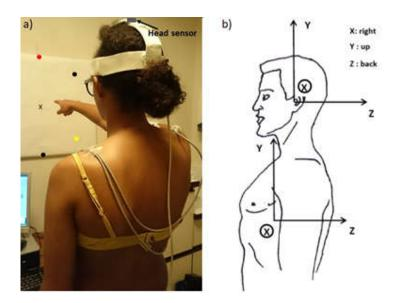
**Figure 1.** Experimental set-up. (**a**) Photo with the helmet (with head sensor) and targets, (**b**) schema of the reference frames.
