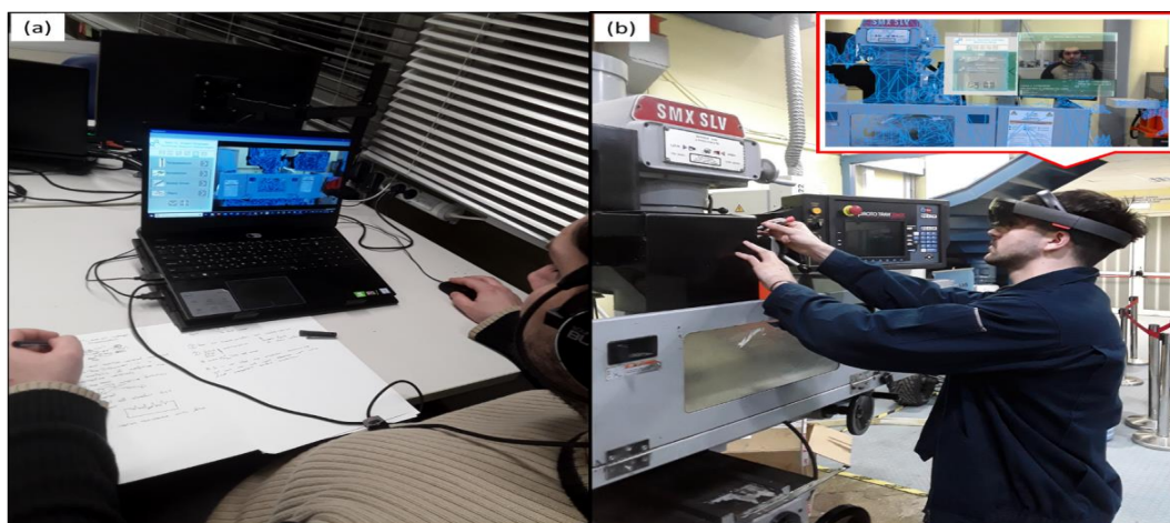
Figure 7. (a) Expert engineer visualizes video stream from technician; (b) Technician is performing maintenance tasks based on expert's instructions.
