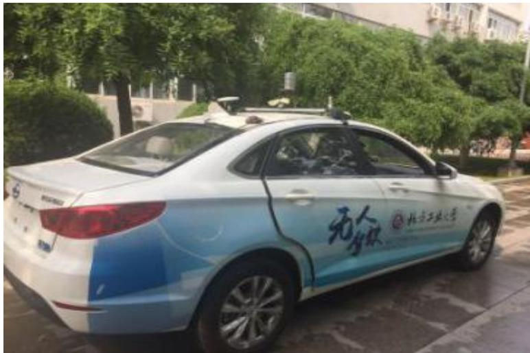
**Figure 6.** Unmanned vehicle platform with light detection and ranging (LiDAR).
