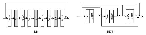
Figure 4. The structure of Residual Block (RB) and Residual Dense Block (RDB).
