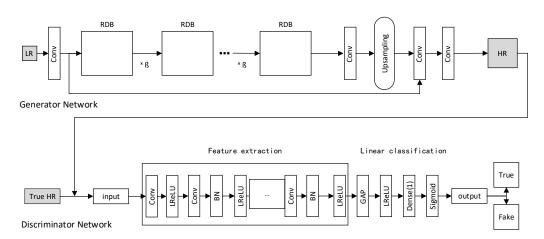
Figure 3. Architecture of generator and discriminator network.
