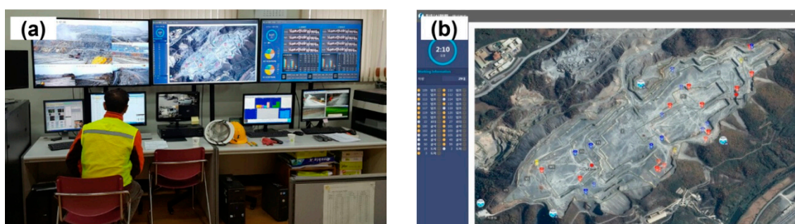
Figure 2. Mine-safety-management system for fleet management of mine equipment: (a) Control center; (b) main dashboard.
