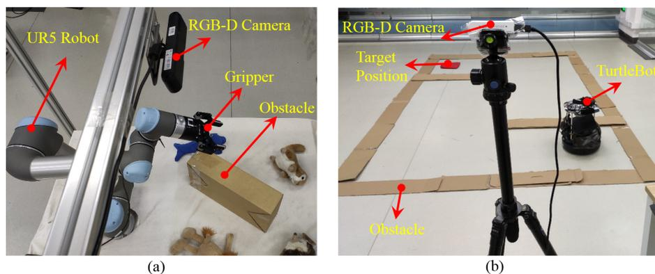
**Figure 4.** Two designated tasks are evaluated for our method. (a) Manipulation task. A policy is trained to control a UR5 robot gripper to reach the target object in 3D space and avoid obstacles (yellow box). (b) Navigation task. Learning a policy navigates the TurtleBot to the target position without obstacle collision.
