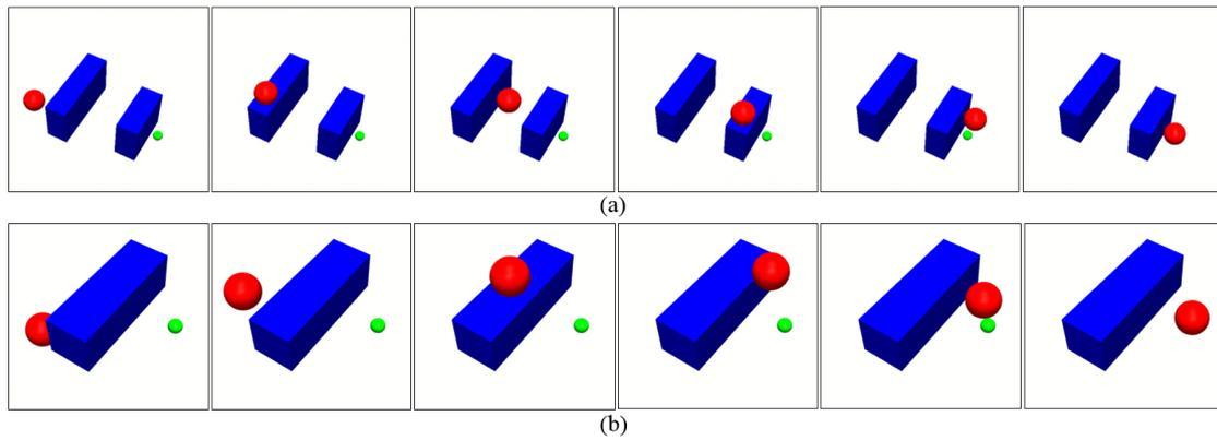
**Figure 8.** Frames captured from the final policies trained with our proposed method deployed on manipulation tasks in simulated environments. (a) two obstacles. (b) one obstacle. Best viewed in color.
