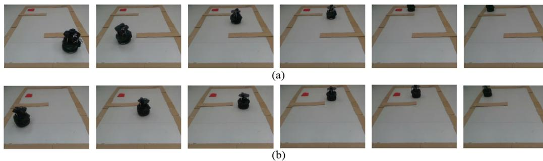
**Figure 11.** Frames of the final policies trained with our method employed on the navigation task in real-world working scenarios. The TurtleBot navigates to the target position without obstacle collision. (a) two obstacles. (b) one obstacle.
