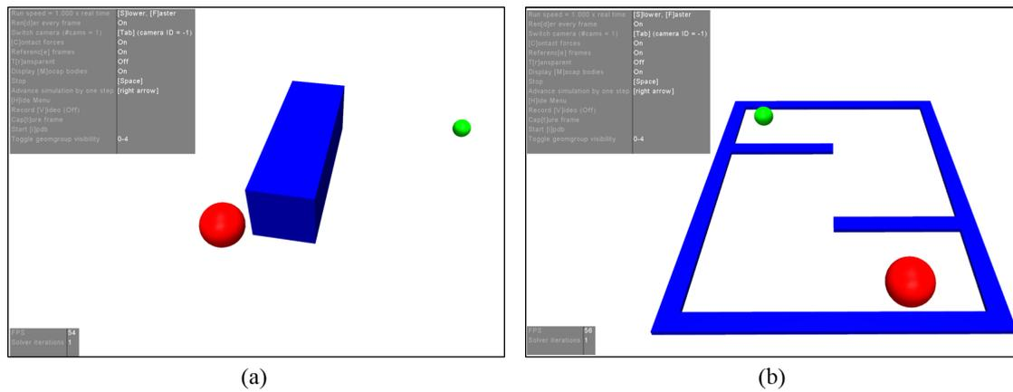
**Figure 6.** Task-relevant simulated environments generated based on our proposed method. (a) Manipulation task. (b) Navigation task. The blue objects are the obstacles, solid red balls are the virtual agents, and green balls denote the target objects (positions). The gray areas illustrate control information of the constructed environment. Best viewed in color.
