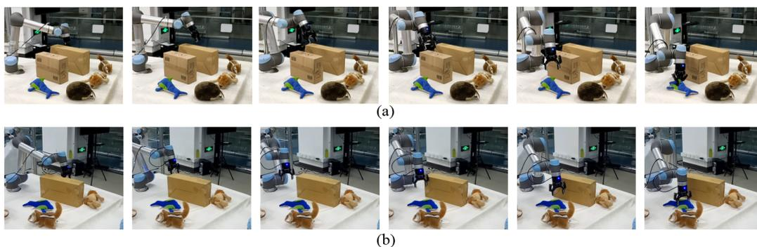
**Figure 10.** Frames of the final policies trained with our method employed on the manipulation task in real-world working scenarios. The robot gripper reaches the target object (toy dolphin) in 3D space and avoiding obstacles. (a) two obstacles. (b) one obstacle.
