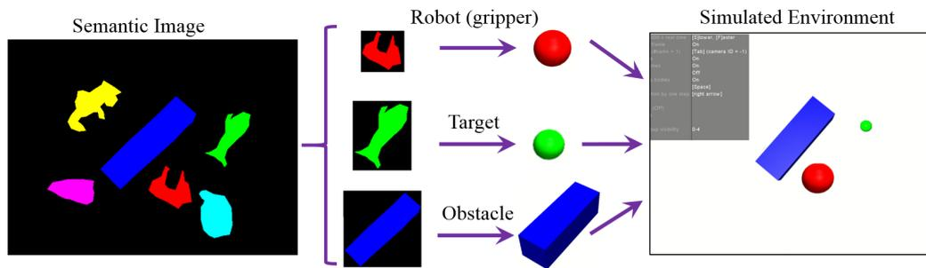
**Figure 2.** Illustration of generating a task-relevant simulated environment. The target object is simplified to its geometry center of the corresponding regions in the semantic image. The robot (or gripper) is equivalent to a solid ball, the center and diameter of which are calculated from its semantic pixel region contour. The obstacles are completely preserved, and other irrelevant objects that cannot be objects are ignored.
