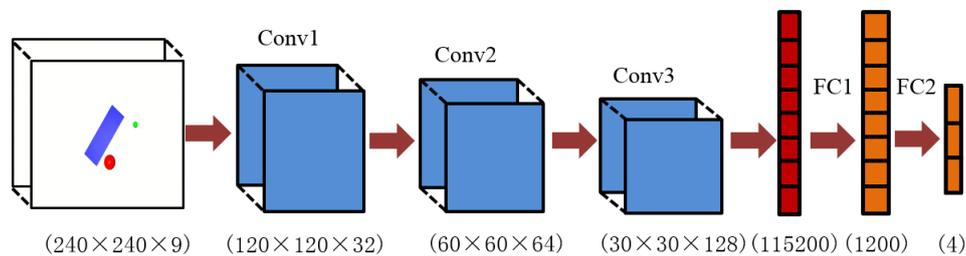
**Figure 3.** Architecture of the designed neural network policy. Two stride steps and a filter size of  $3 \times 3$  are used for all three convolution networks. The ReLU nonlinear activation function is used throughout, with no pooling and no dropout techniques applied. The input is three RGB images from a simulated environment downsized to ( $240 \times 240$ ) with 9 channels, and the output is action.
