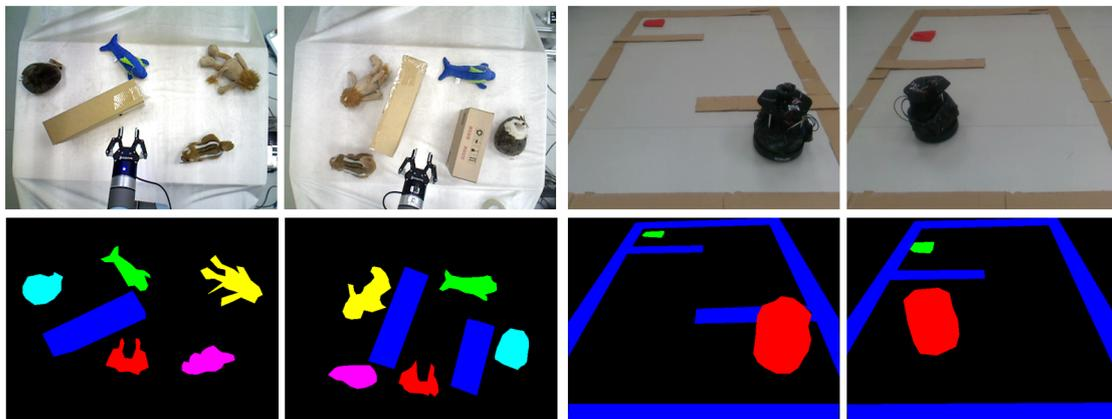
**Figure 5.** Semantic segmentation results of robot working scenarios. The first row shows the RGB images, and the second row shows their corresponding semantic images. The left two are for the manipulation task, and the right two are for the navigation task. Best viewed in color.
