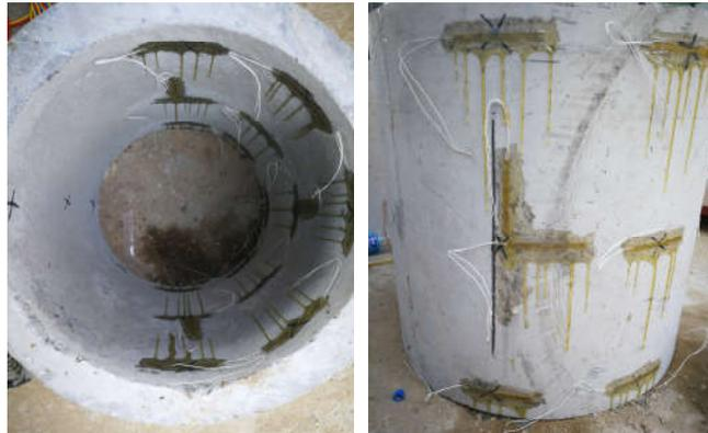
**Figure 7.** Gluing strain gages in position.
