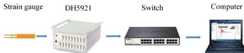
**Figure 8.** Data acquisition process.
