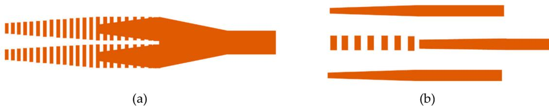
**Figure 9.** Schematic of (a) fork-shape coupler and (b) trident coupler assisted with subwavelength gratings structure.
