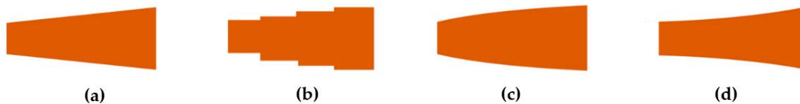
**Figure 3.** Schematic of the (a) linear; (b) multi-sectional; (c) parabolic; and (d) exponential Si inverse tapers (top view).
