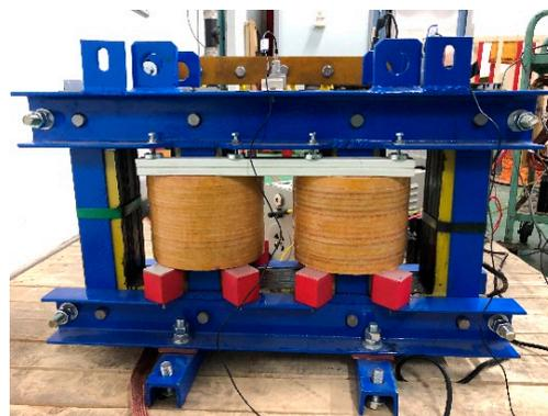
**Figure 2.** Reduced-scale autotransformer.
