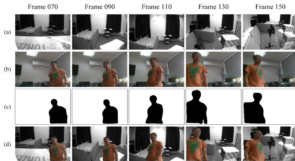
Figure 10. The processing of the V202_syn sequence. (a): Images in original Euroc V2_02 sequence. (b): Images collected by ourselves, containing a pedestrian. (c): Sematic images obtained by Mask-RCNN. (d): Images in the modified V202_syn sequence.
