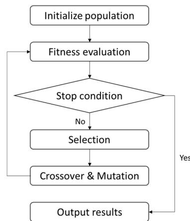
Figure 5. Genetic algorithm procedure.
