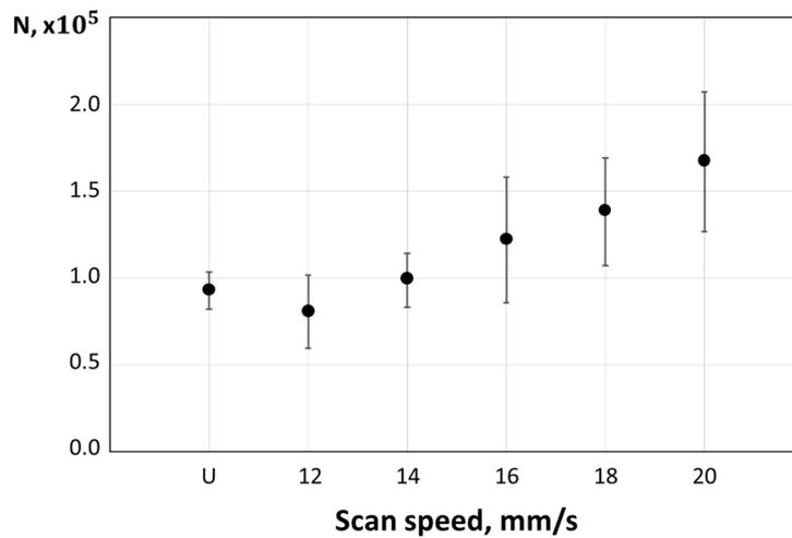
**Figure 8.** Number of cycles vs. scan speed for a laser power of 200 W. ‘U’ refers to the untreated samples.
