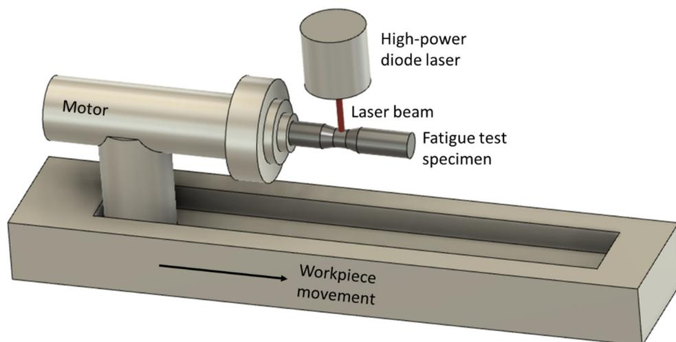
**Figure 2.** High-power diode laser system.
