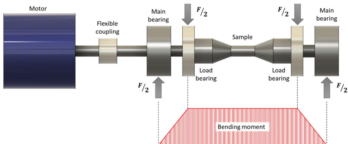
**Figure 3.** Schematic representation of the four-point rotating bending machine.
