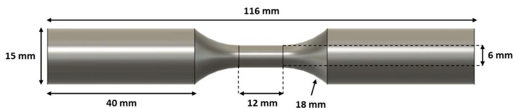
**Figure 1.** Geometry of the samples obtained according to ASTM E466.
