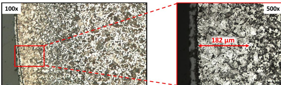
**Figure 9.** Optical micrography of a laser hardened cross-section: transition from the martensitic structure (light grey) to the ferrite and perlite structure (dark grey) for  $P = 200$  W and  $S_s = 20$  mm/s.
