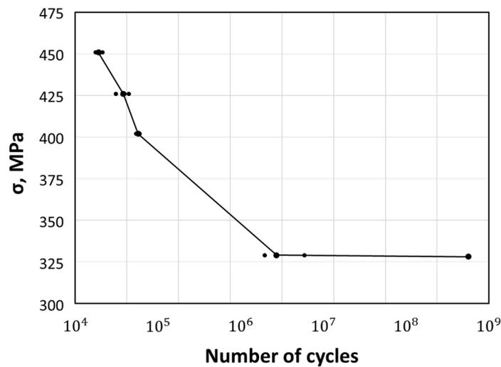
Figure 4. Wöhler curve for the untreated samples.
