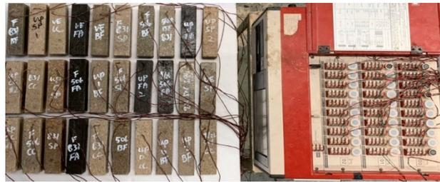
**Figure 4.** Test setup for measuring drying shrinkage.
