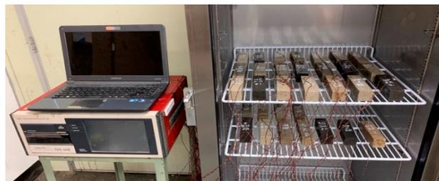
**Figure 5.** Test setup for measuring thermal expansion.
