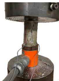
**Figure 3.** Test setup for determining the modulus of elasticity.
