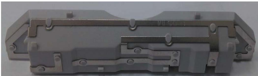
**Figure 2.** Fabricated PIFA.
