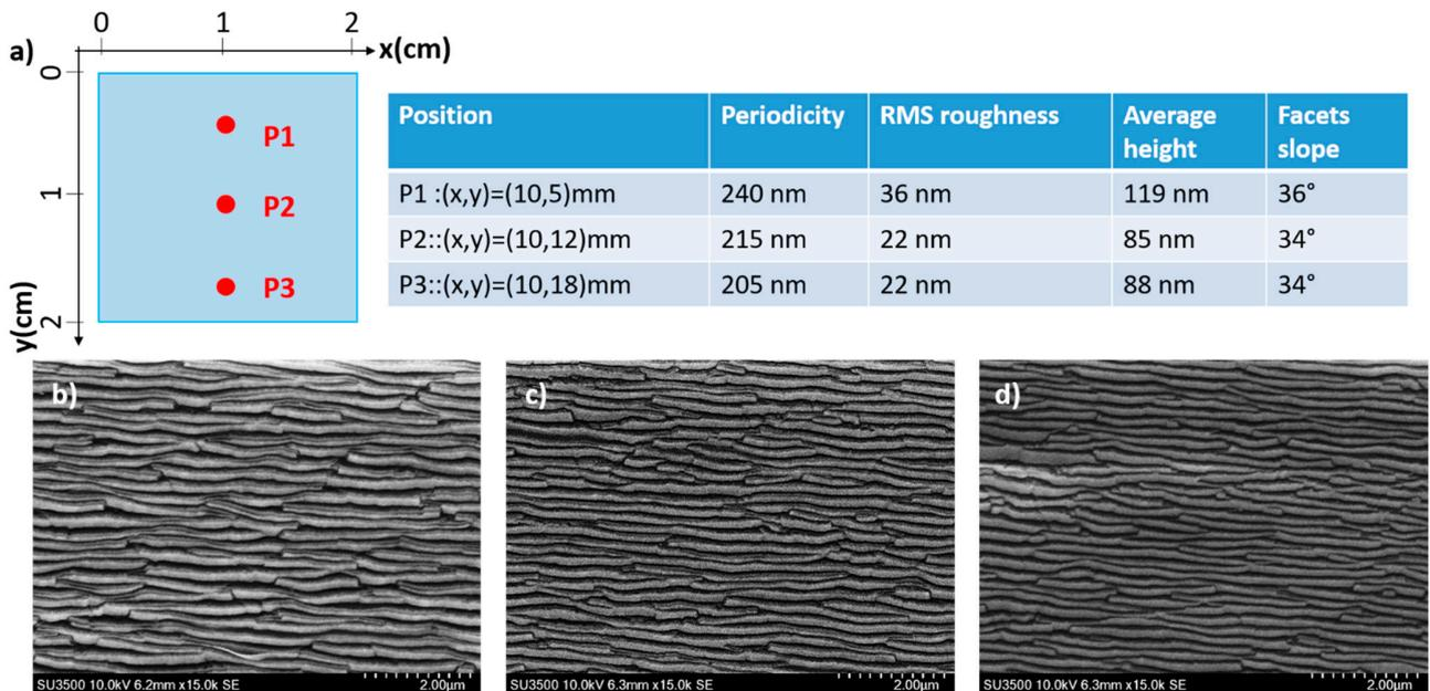
**Figure SI2 (a)** Sketch of the sample where are highlighted the regions P1, P2 and P3 characterized by AFM microscopy (see characteristic parameters in the table. **(b-d)** SEM images of Au nanostripe arrays confined in region P1, P2 and P3 respectively. The images clearly highlight the large area homogeneity of these plasmonic templates.
