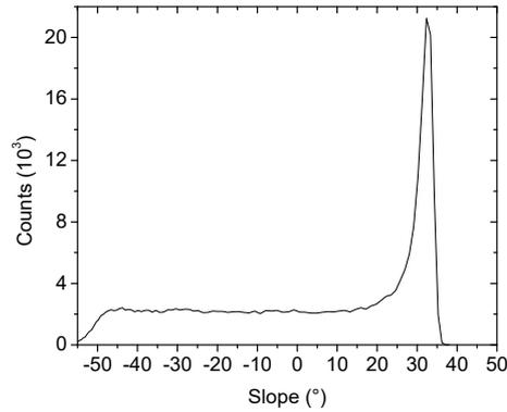
**Figure SI1** Histogram of the slope distribution of a typical rippled glass template.
