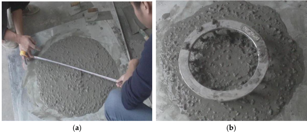
Figure 3. The basic workability test of S_0 SCC. (a) Slump flow test (SF = 700 mm); (b) J-ring test (SF J = 670 mm).
