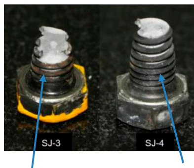
(a) Bending failure Tensile failure
