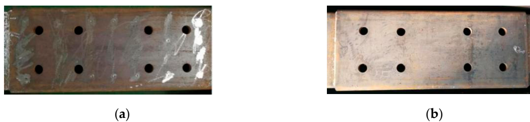
Figure 3. Connection mode of the C-channel. (a) With plug welding and (b) Without plug welding.
