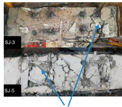
(b) Local concrete crush
