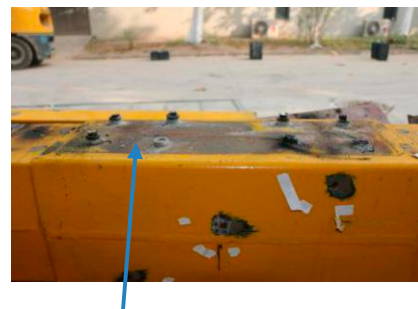
(f) Slight outward deformation
