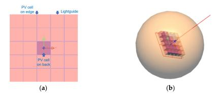
**Figure 3.** The geometry of the LSC PV device shown in Case 3 of Table 1: (**a**) top view of device; (**b**) the orange sphere shows the diffuse irradiance and the red line indicates the direction of the direct beam irradiance.
