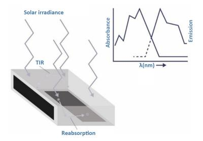
**Figure 1.** The design and working principle of a luminescent solar concentrator photovoltaic (LSC PV) element, with solar cells attached to the edges, showing the absorption spectrum (solid line) and the emission spectrum (dotted line) of a dye in an LSC.
