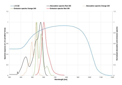
**Figure 4.** The quantum efficiency curve of a silicon solar cell versus the normalized absorption and emission spectra of the Lumogen red 305 and orange 240 dyes.
