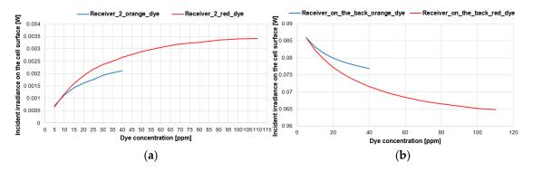
**Figure 6.** A comparison of the direct incident irradiance on the solar cells in LSC PV design Configuration 2—see Table 1—under exposure to standard test conditions (STC) irradiance (1000 W/m<sup>2</sup>, 100% direct) for the case of the orange and the red dyes: (**a**) the solar cell surface in between the lightguides; (**b**) the solar cell surface at the back.
