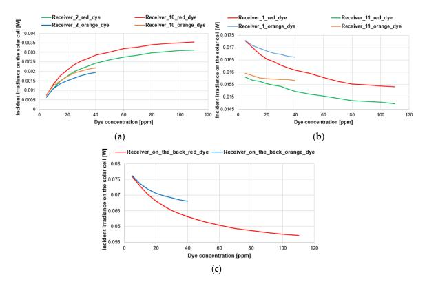
**Figure 7.** A comparison of the diffuse incident irradiance on the solar cells in LSC PV design Configuration 2—see Table 1—under exposure to STC irradiance (1000 W/m<sup>2</sup>, 50% direct and 50% diffuse) for the case of the orange and the red dyes: (**a**) the solar cells surface in between the lightguides, inner sides; (**b**) the solar cell surface in between the lightguides, outer sides; (**c**) the solar cell surface at the back.
