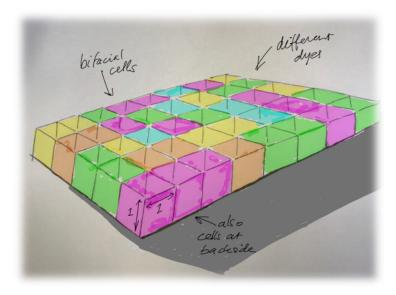
**Figure 2.** A sketch of a bifacial LSC PV mini-module for building-integrated PV (BIPV) applications by Ned Ekins-Daukes and Angèle Reinders, made during the Exciton Solar + Design Summer School at the University of New South Wales (UNSW), Sydney, 2019.
