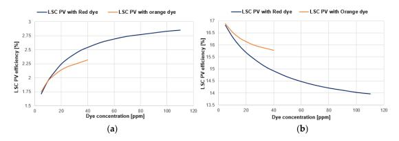
**Figure 8.** The efficiency of the LSC PV devices as a function of the dye concentration: (**a**) the device with the cells on the edges (case 3); (**b**) the device with the cells on the back and on the edges (case 5).
