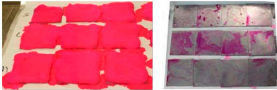
Figure 5. Residual staining after the application of TBF 300 on coupons where microbial biofilms were grown for 10 days. Each row corresponds to biofilms of different microorganisms: Salmonella spp. ( upper row ), L. monocytogenes ( central row ), mixed biofilm ( lower row ).
