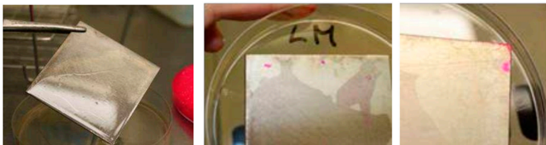
Figure 4. Residual staining after application of TBF 300 on a coupon where a L. monocytogenes biofilm was grown for 3 days.
