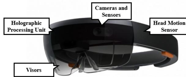
Figure 2. The mixed reality device HoloLens.
