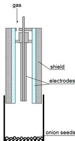
**Figure 1.** Schema of experimental set up with radio frequency atmospheric pressure plasma jet.
