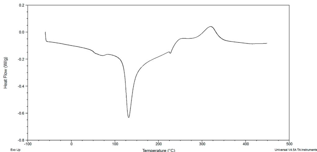
**Figure 1.** Differential scanning calorimetry (DSC) curve of coffee silverskin sample.
