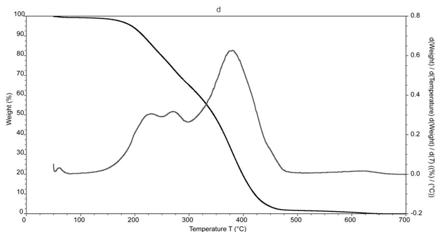
**Figure 2.** (a) Thermogravimetry/derivative thermogravimetry (TG/DTG) curves of coffee silverskin in oxygen atmosphere. (b) TG/DTG curves of coffee silverskin in nitrogen atmosphere. (c) TG/DTG curves of coffee silverskin fat samples in oxygen atmosphere. (d) TG/DTG curves of coffee silverskin fat samples in nitrogen atmosphere.
