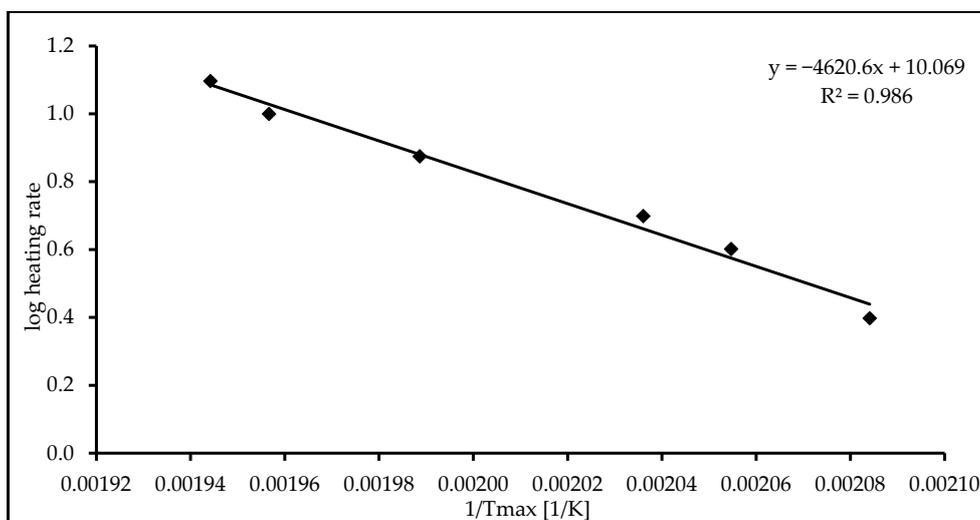
**Figure 5.** Temperature shift at the maximum (of the oxidation process) of DSC curves depending on the logarithm of heating rate of the thermo-oxidative decomposition of silverskin fat.
