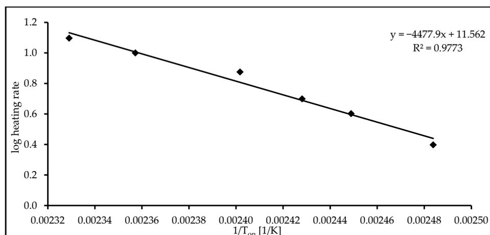
**Figure 4.** Temperature shift at the onset (of the oxidation process) of DSC curves depending on the logarithm of heating rate of the thermo-oxidative decomposition of silverskin fat.
