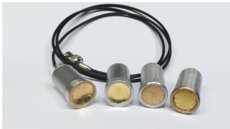
Figure 2. Picture of transducer prototypes, from left to right: HS03 focused (radius of curvature: 22 mm), HS03 focused (radius of curvature: 35 mm), HS06 flat, HS03 flat.
