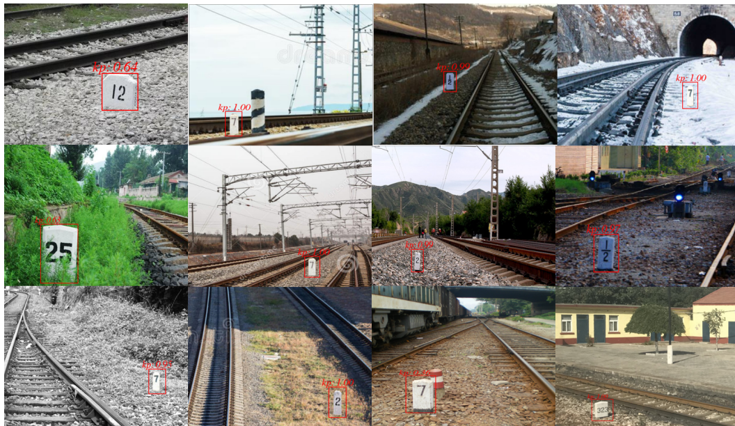
Figure 9. Detection and location results of kilometer post (kp).
