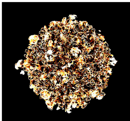
(c) MAUI/LUX image of a 15 kg Comp B fireball
