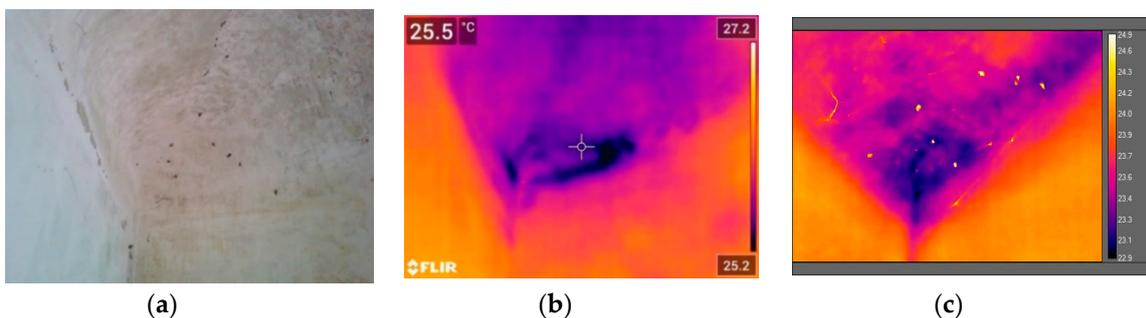
Figure 4. (Left to right) the set of images represent adjacent inside corner of the lower ground oval eastern room area. (a) Is the visual image of the area, (b) is the thermal image taken during the survey in August 2019, (c) is the thermal image taken during the survey in February 2020.
