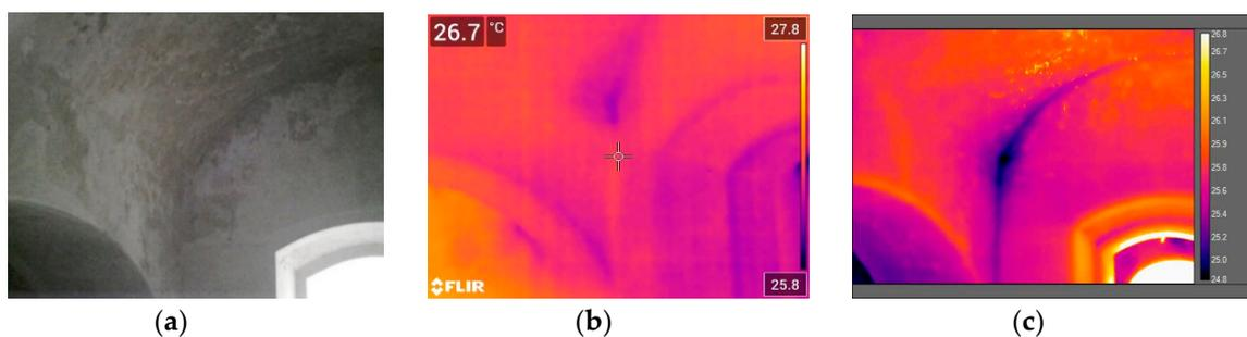
Figure 3. (Left to right) the set of images represent the left corner of the eastern arch in the lower ground oval eastern room. (a) Is the visual image of the area, (b) is the thermal image taken during the survey in August 2019, (c) is the thermal image taken during the survey in February 2020.
