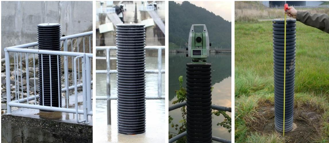
**Figure 1.** An example of an inappropriately stabilized measurement pillar.
