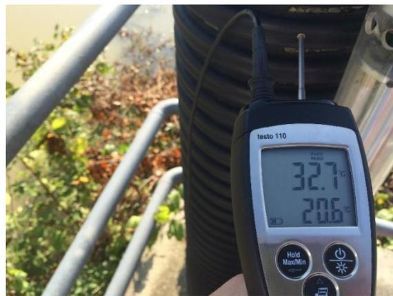
**Figure 2.** Temperatures measured on the sunny and shady side of the measurement pillar.
