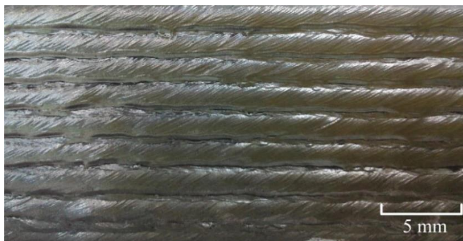
Figure 12. Surface topography of a specimen manufactured by wire arc additive manufacturing (WAAM). Reproduced from [141] (Open access, no copyright).
