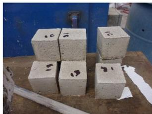
(a) Compression test probes: 0.05 × 0.05 × 0.05 m
