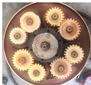
Figure 24. Spur gear failure in a ball-milling machine.
