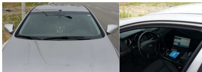
Figure 11. Experimental setup for steering pull measurement.
