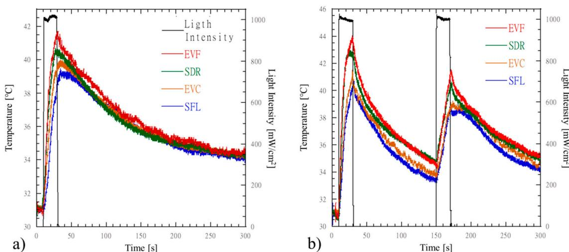
**Figure 3.** Simultaneous time measurements of temperature and photo-diode signals for MOD cavities restored with the investigated bulk-fill RBCs according to: (a) the bulk-fill technique; (b) the incremental technique.
