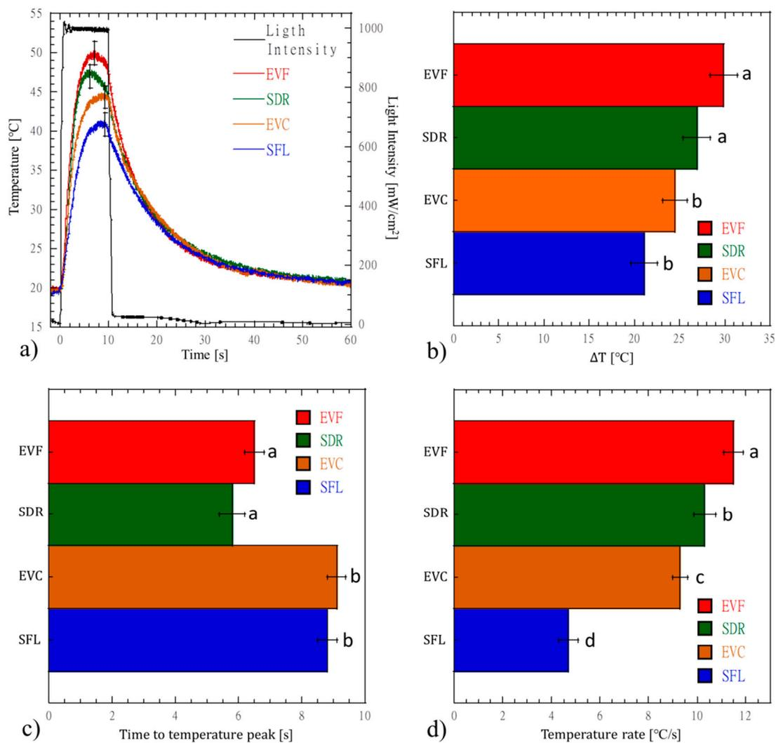
**Figure 2.** (a) Temperature profiles developing into bulk-fill RBC; (b) maximum temperature rise; (c) time to temperature peak; and (d) temperature rate. Error bars represent the standard deviation. Different letters reported beside the bars indicate a significant difference between the means ( $p < 0.05$ ).
