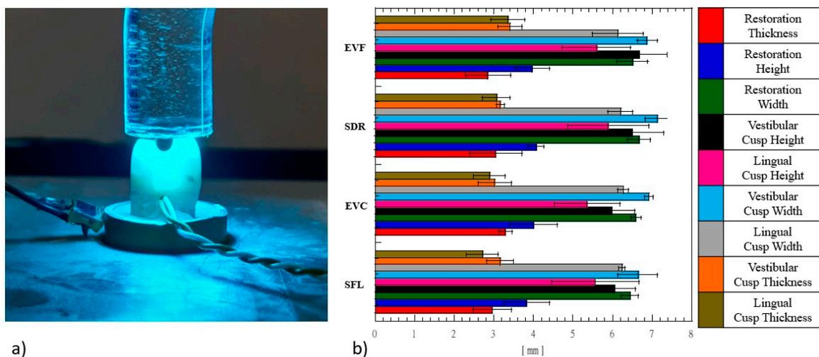
**Figure 1.** (a) Experimental set-up for the simultaneous measurement of light intensity and temperature levels occurring in mesio-occlusal-distal (MOD) cavities; (b) geometrical details of human premolars and MOD cavities (b).
