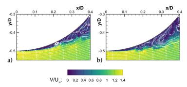
**Figure 10.** Instantaneous velocity magnitude and streamlines at  $\text{Re} = 1.69 \times 10^5$ , showing the intermittency of the separation bubble (equivalent bowling speed of 78 mph).
