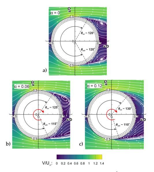
**Figure 12.** Time-averaged velocity magnitude in the *x*-*z* plane at Re =  $1.94 \times 10^5$  (U<sub> $\infty$ </sub> = 20 m/s) showing (a) the symmetric flow field with no rotation and (**b**,**c**), the Magnus effect demonstrated at two different spin rates. Separation angles shown to nearest 5°.
