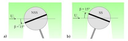
Figure 7. Position of the ball to investigate (a) the non-seam side (NSS) and (b) the seam side (SS).
