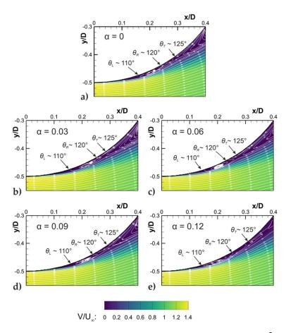
**Figure 11.** Time-averaged velocity magnitude and streamlines at Re =  $1.69 \times 10^5$  on the NSS for different spin rates,  $\alpha$  (equivalent bowling speed of 78 mph). Separation and reattachment angles shown to nearest 5°.
