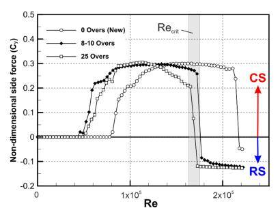
**Figure 3.** Variation of non-dimensional side force ( $C_y$ ) with Reynolds number (Re) for Dukes balls at different stages of wear, showing the transition from CS to RS. The double-sized ball used in this paper is comparable in surface roughness to the 25-over-old ball. The critical region for the 25-over-ball is highlighted ( $1.65 \times 10^5 < \text{Re}_{\text{crit}} < 1.75 \times 10^5$ ). Adapted from [4].
