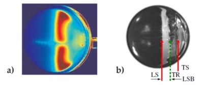
**Figure 4.** Evidence of a laminar separation bubble on the NSS using two different methods: (**a**) heat flow method on a double-sized cricket ball model [5] and (**b**) oil flow visualization on a sphere with a trip [14].
