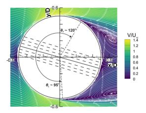
**Figure 8.** Time-averaged velocity magnitude and streamlines at  $U_{\infty} = 12 \text{ m/s}$ , Re =  $1.1 \times 10^5$  (equivalent bowling speed of 54 mph), showing conventional swing, on the seam side  $\theta_{\text{T}} \sim 120^\circ$  and on the non-seam side  $\theta_{\text{L}} \sim 95^\circ$ . Separation angles shown to nearest 5°.
